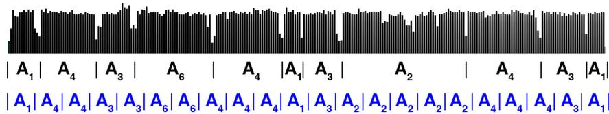
**Fig. 1.** Partitioning of raw sensor signal into separate activities  $A_1$  to  $A_6$  with Def. 1, HAR problem (black) and fixed window size, relaxed HAR problem (blue).
